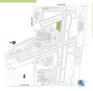
Two dedicated aircraft deicing pads are included to enhance safety during winter weather conditions and to manage the handling of aircraft deicing fluids more efficiently. During non-deicing conditions these pads will also be used to hold aircraft diverted to, or parked at, MKE overnight or for an extended duration.
