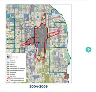
Since MKE's Part 150 Noise Study was completed in 2009, there has been notable industry change relative to aircraft noise. Significantly, advancements in aircraft airframe and engine technology, evolution of the overall aircraft fleet, and air traffic changes have all reduced the noise footprint associated with aircraft operations at MKE. As a consequence, aircraft noise exposure in the vicinity of MKE is significantly less than was predicted and simulated in the Airport's Part 150 Noise Study.
